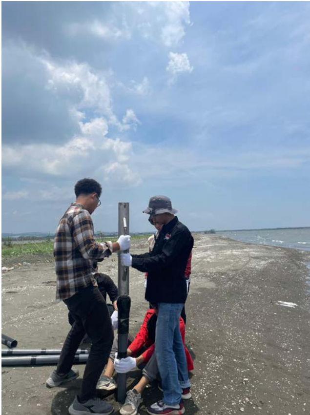
Fig. 2. Gravitational coring sample collection and field conditions of the longshore bar.
